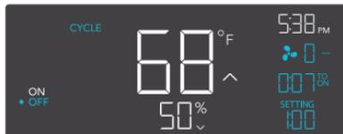
If there is a speed set in OFF Mode other than zero, the fans will run at that speed when triggered to turn off.
